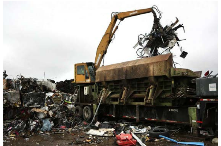
A baler operator lifts light-gauge ferrous materials into a baler at Texas Disposal Systems' landfill in Creedmoor just south of Austin. TDS' focus has been on diversion, and they've spun off 13 businesses from their landfill operation.
